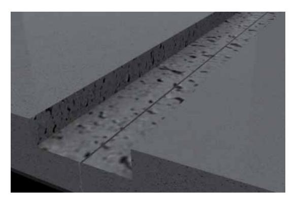
Put also special primer on all sides of the concrete slab for good adhesion of filling substance. Drill some holes in the concrete bottom positioned at the same distance as the anchorage of the HC-Sinus Slide® repair joint. Install screwed rod trough the anchorage openings and fix into the drilled holes. Level out the HC Sinus Slide® joints down and across.
